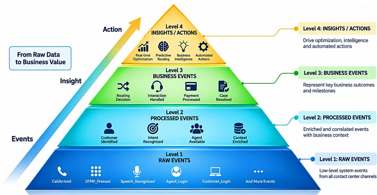
Figure 3.4. Event-Driven Contact-Center Architecture from Raw Events to Insights and Automated Actions
