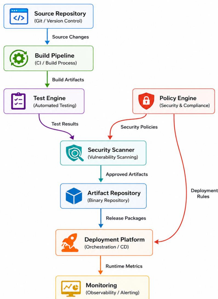
Figure 28: Automated DevSecOps Security Validation and Secure Deployment Pipeline
